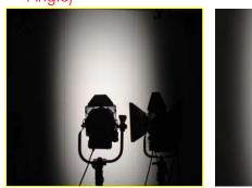
The Barndoor in a NOT REAL FRESNEL optics does not work properly: the projection is OVAL and the more you barndoor the more you dim the central beam
