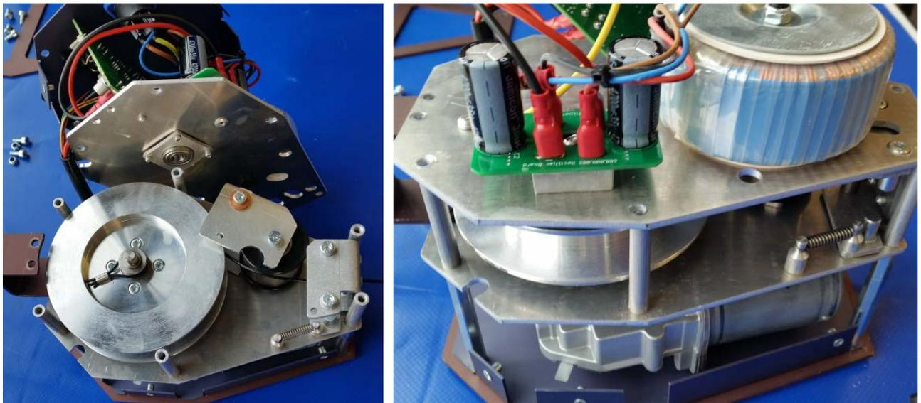
18. Tighten the bolts and nuts for the mounting bracket. Check that you use the right bolts, by ensuring that the bolt goes through the nut and self-locks.
