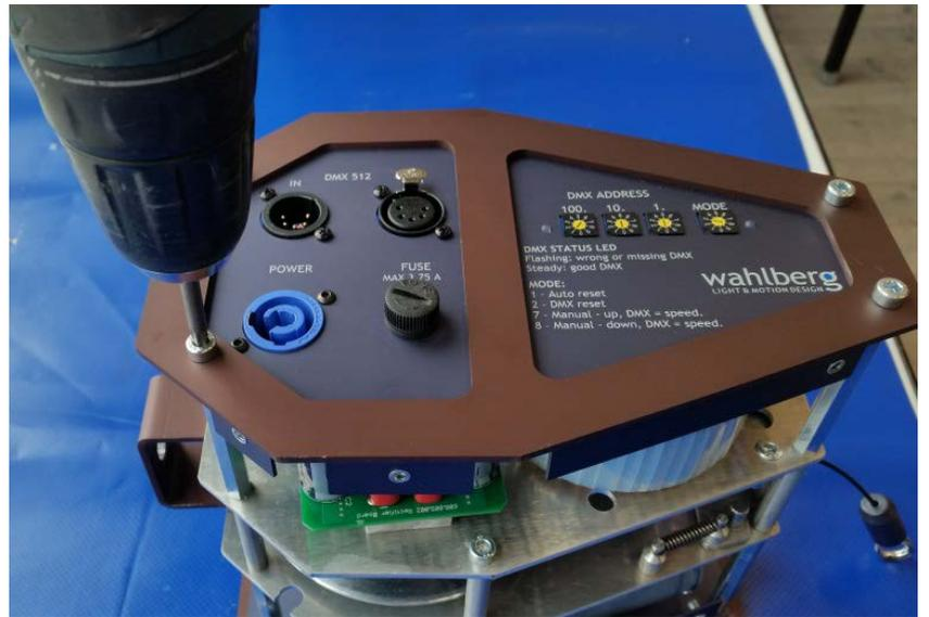
6. Remove the four hexagonal spacers and the two bolts holding the TRAF0-plate.
