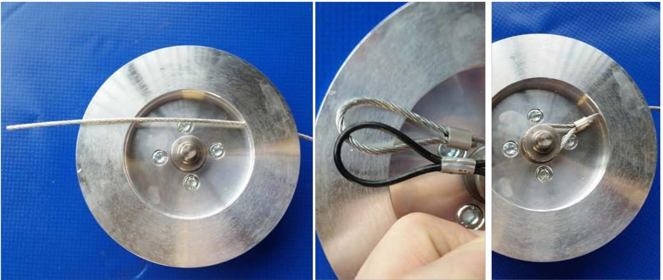
15. Mount the wire-wheel back on the winch. You might need to take out the slack detection to make it fit in.
