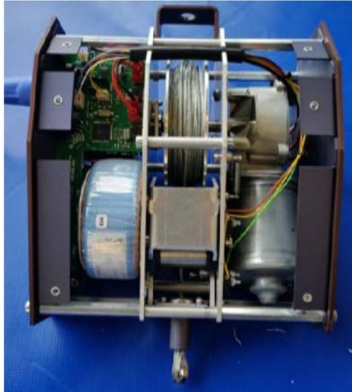
4. If the wire is not tight around the wire-wheel, or it is bungled up inside, the wire needs to be unravelled.
