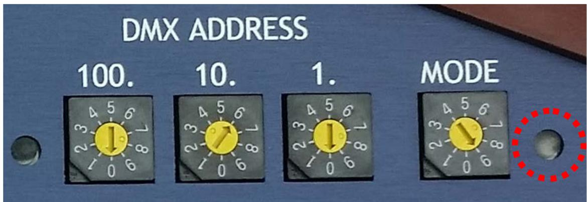
The position is set on the DMX channel 1 and 2, which controls the rough-and fine-position. Where 100 % is the soft TOP limit and 0 % is the soft BOTTOM limit.
